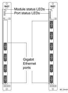
Figure 1-5: G4X module and G6X module
