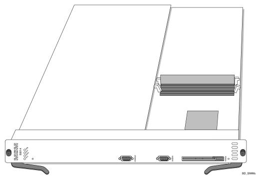
Figure 1-4: MSM DIMM sockets
