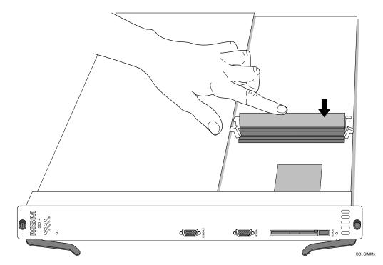
Figure 3-3: Adding a DIMM
