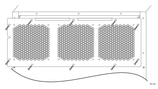
Figure 3-2: Removing the fan tray
