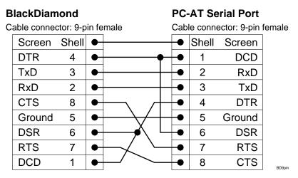
Figure 2-6: PC-AT serial null-modem cable pinouts
