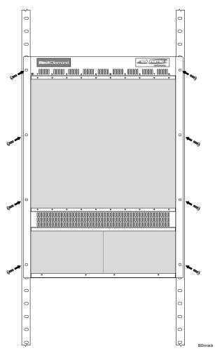
Figure 2-2: BlackDiamond chassis mounted in rack
