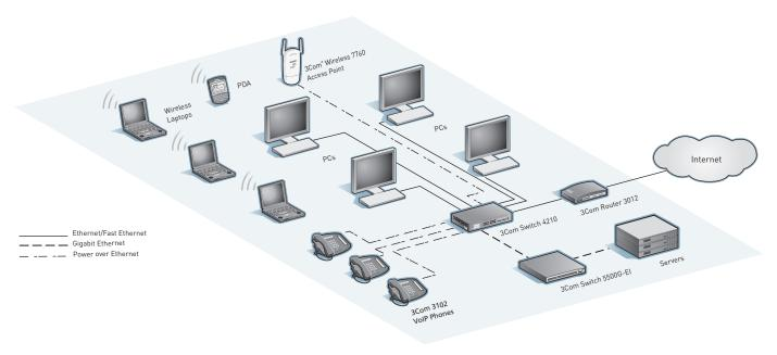
In the above network, 3Com Switch 4210 and Switch 5500G-EI units are managed as a single cluster.
