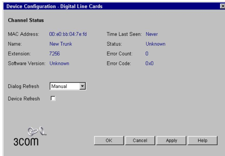
**Figure 136** Channel Status Dialog Box — T1 ISDN PRI
