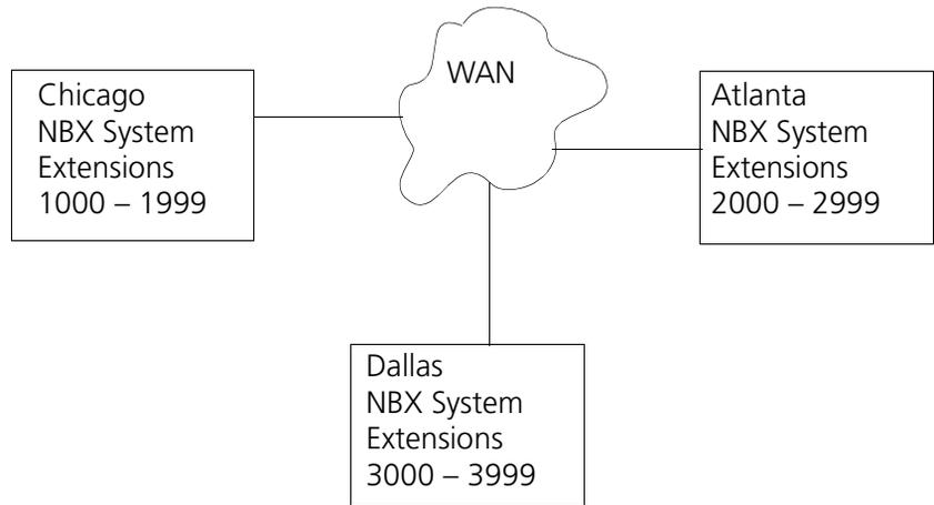
In the sample network shown in [Figure 28](#), each site is set up to use a unique range of telephone extensions. The dial plan on each of the systems is configured so that whenever a call is made to an extension not located at the local site, the NBX system sets up a VTL connection to the appropriate site.
