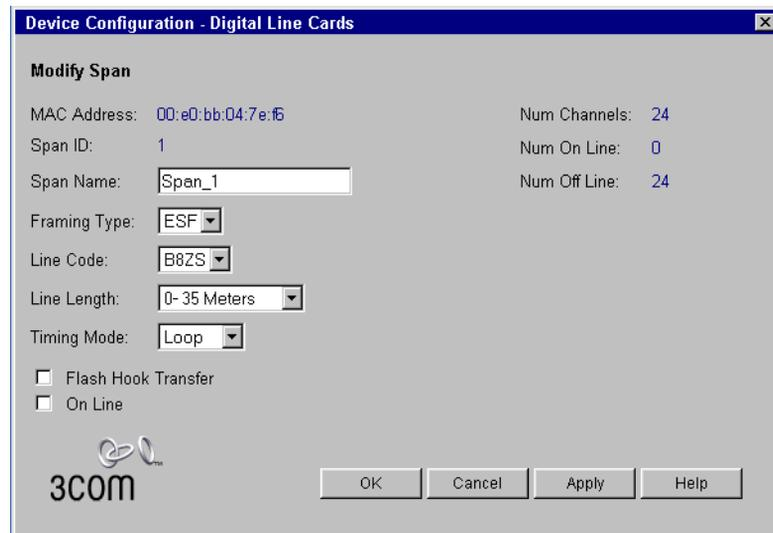
**Figure 127** Modify Span Dialog Box — ISDN PRI
