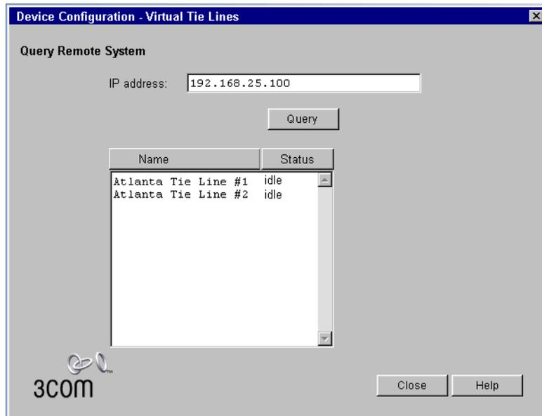
The Atlanta system (IP address 192.168.25.100) shows two installed but idle VTL connections. If you performed the Query Remote test from the Atlanta office and specified the IP address of the Chicago system, it should show two installed but idle VTL connections.
