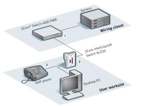
IEEE 802.3af-compliant Power over Ethernet network configuration with power forwarding to another device:
