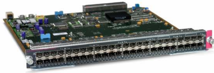
Figure 1. Classic 48 Port 100BASE-X Fiber Interface Module (part number WS-X6148-FE-SFP)
