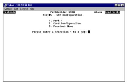
**3** Select [1] Port 1 to open the SIM Port Configuration Port/LMI selection menu, shown in Figure 86.
