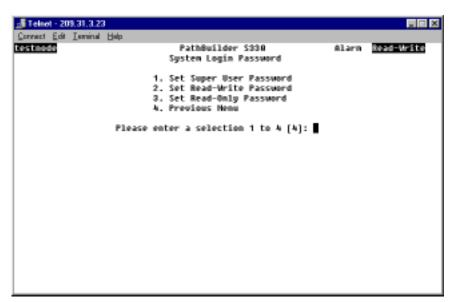
3 Select [1] Set Super User Password, [2] Set Read-Write Password, or [3] Set Read-Only Password to set the desired password.
