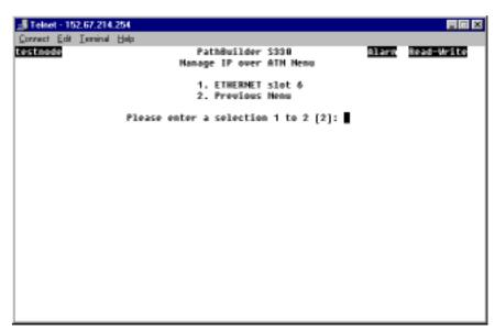
**c** Enter the number corresponding to the Ethernet port for which you want to configure IP over ATM. The IP over ATM menu for the selected port appears, as shown in Figure 102.
