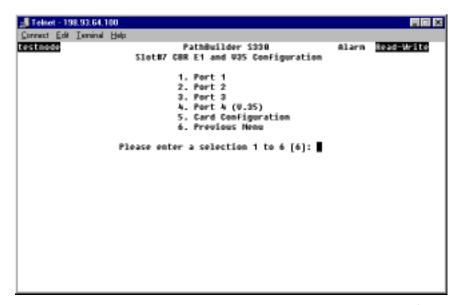
**3** Select the option corresponding to the port you want to configure ([1] Port 1, [2] Port 2, or [3] Port 3). The CBR T1-DSX/E1Port Configuration menu for the selected port appears. Figure 110 shows a CBR Port Configuration menu for an CBR E1 card.
