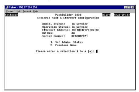
Figure 90 Ethernet Configuration Menu
