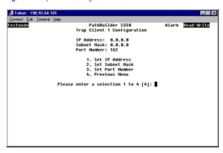
**3** Enter the following information (by selecting the appropriate options and responding to the prompts that appear at the bottom of the screen) to configure the trap client:
