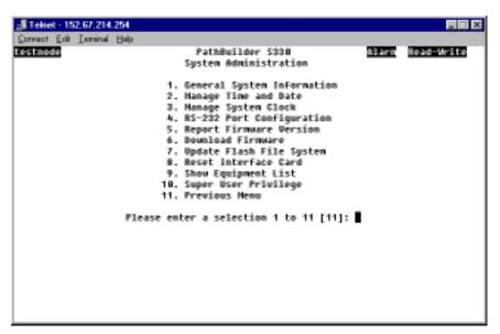
**2** From the System Administration menu, select [3] Manage System Clock to open the System Clock Configuration menu, shown in Figure 41.
