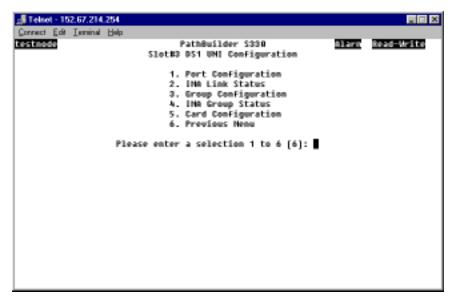
3 Select [1] Port Configuration to open the T1 (DS1)/E1 UNI Port Configuration Selection menu. Figure 68 shows the T1 (DS1) UNI Port Selection menu. The E1 UNI Port Configuration menu is the same.
