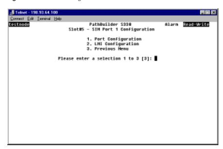
**4** Select [1] Port Configuration to open the SIM Port Configuration menu, shown in Figure 87. This menu displays the current serial port configuration and provides options that allow you to change certain parameters.
