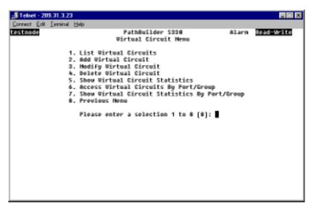
2 Select [2] Add Virtual Circuit. The Add Virtual Circuit screen appears as shown in Figure 120.
