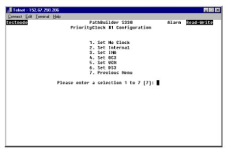
**b** Enter the option number corresponding to the clock source you want to designate as the priority 1 (highest priority) system reference clock to open the Reference Clock Selection menu for that interface. Figure 43 shows the OC3 Reference Clock Selection menu. The menus for the other interfaces are similar.
