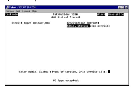
**3** Set the administrative status for the circuit. A screen appears, listing the PathBuilder S330/S310 modules and ports by slot number and prompting you to select a slot for side A, as shown in Figure 124.
