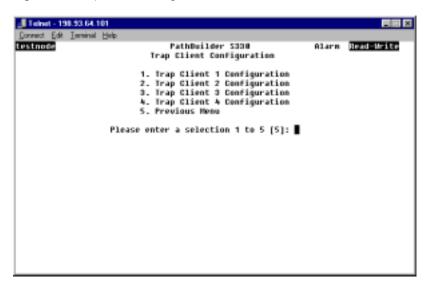
**2** Select the number corresponding to the trap client you want to configure. Figure 49 shows the menu for configuring trap client 1.
