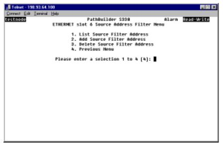
2 Select [2] Add Source Filter Address. The Add Source Address Filter screen appears. This screen displays the following prompt:
