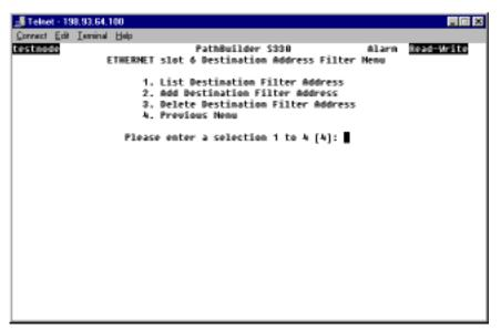
2 Select [2] Add Destination Filter Address. The Add Destination Address Filter screen appears. This screen displays the following prompt:
