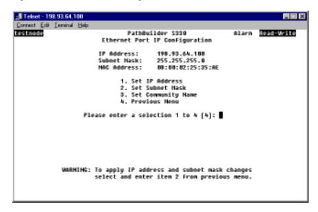
**3** Enter the following information (by selecting the appropriate options and responding to the prompts that appear at the bottom of the screen) to set local host interface parameters:
