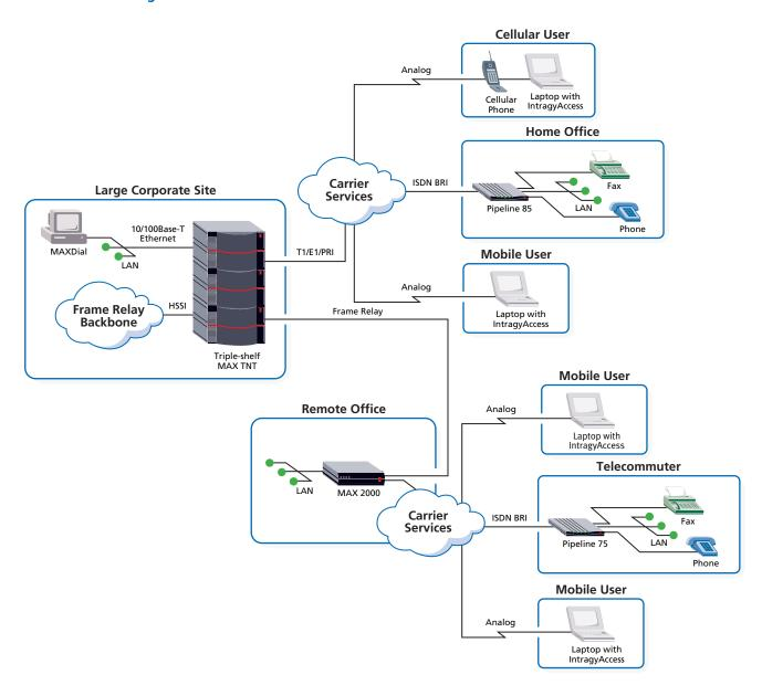
The MAX TNT allows corporate users to connect to a single high-density platform that supports 720 remote connections and up to 150 T1/E1 Frame Relay connections. Up to 720 of the remote connections can be analog or cellular modem users.
