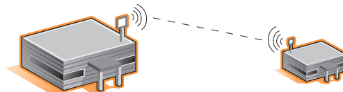
Figure 2. Point-to-point connections from one building to another using sector panel antennas.
